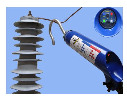
Arrestor test with the ADD™
