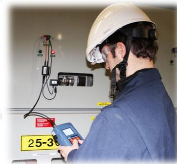
Bi-Phase coupler used on a switchgear with XDP-II™ partial discharge detector
